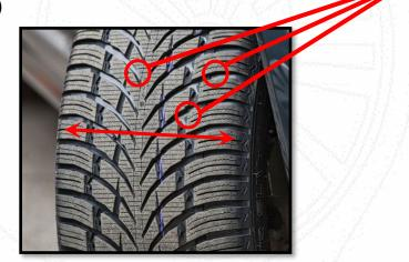
Info: If you pay attention to small elevations in the tread grooves, the socalled <u>Tread Wear Indicator</u>, you can determine the height of 1.6mm.
